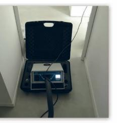
After laying the ducts, the companies perform a smoke test as a self-test. After the laying, the phases of dressing of the columns can generate duct breaks.
