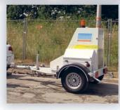
> After the dynaplaque Type II, Rincent ND Technologies produces an equipment FWD-HWD (Falling Weight Deflectometer and Heavy Weight Deflectometer). This equipment is carried by a chassis respecting the prevailing European standards.
