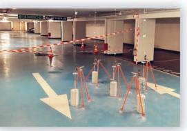
The loading test is carried out in steps, the last being of 24 hours. The deflection is measured vertically to the load, in this case on the lower level, at several points by means of tensioned invar wires, associated with digital comparators accurate at 0.02mm.
