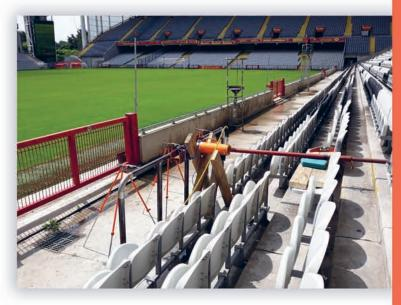
The stair steps of the bleachers were used to mobilize the response to the force measured by a calibrated and verified load cell.
